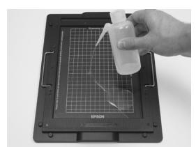
2. Place film on top of the KAMI applied area and align with grid in Mounting Station.
