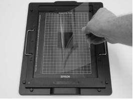
5. Air Bubbles should not be present in the image area. If air is present take a Scanner Wipe and wipe AZ-42 to remove bubbles.
