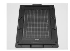
1. With KAMI SMF Optical Fluid in the Application Bottle lightly spray the area of the holder where the film will be placed.
