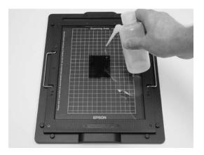
4. Take a pre-cut sheet of AZ-42 Optical Mylar and roll from left to right over the Mounting Bed.
